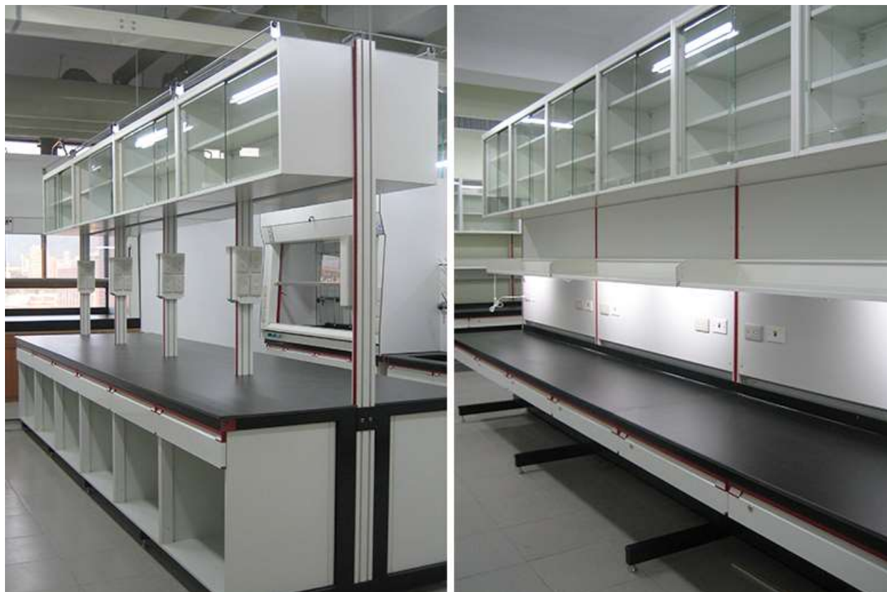
A typical Labaire installation with suspended cabinets (drawer and sliding glass door cupboard), black anodized aluminium framework, black Phenolic Resin worktops, natural anodized extruded aluminium extensions with electrical services and over bench cabinets. Specialised shelving is installed in this application.
